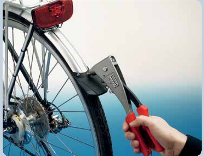
Easy riveting of protection plates
